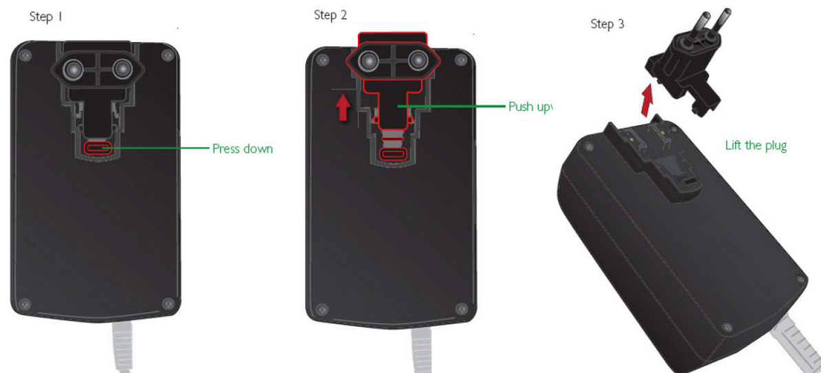
Image 6: Assembly of primary plug (Image courtesy of FRIWO Gerätebau GmbH, Germany)
